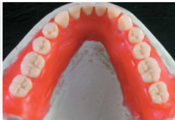
Fig. E Transfer the new denture set-up and wax-up onto the duplicate model and complete final wax modeling.
